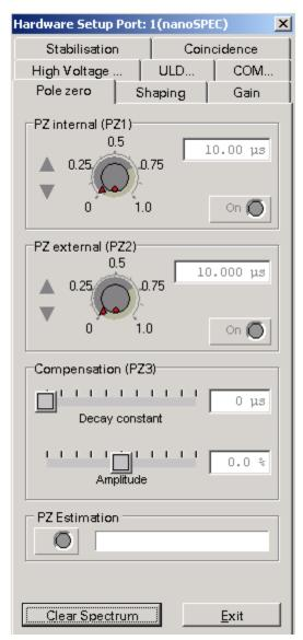
You determine the decay constant of the internal differentiation stage by specifying **PZ INTERNAL** (PZ1). This value is preset by manufacturer and should not be changed.
