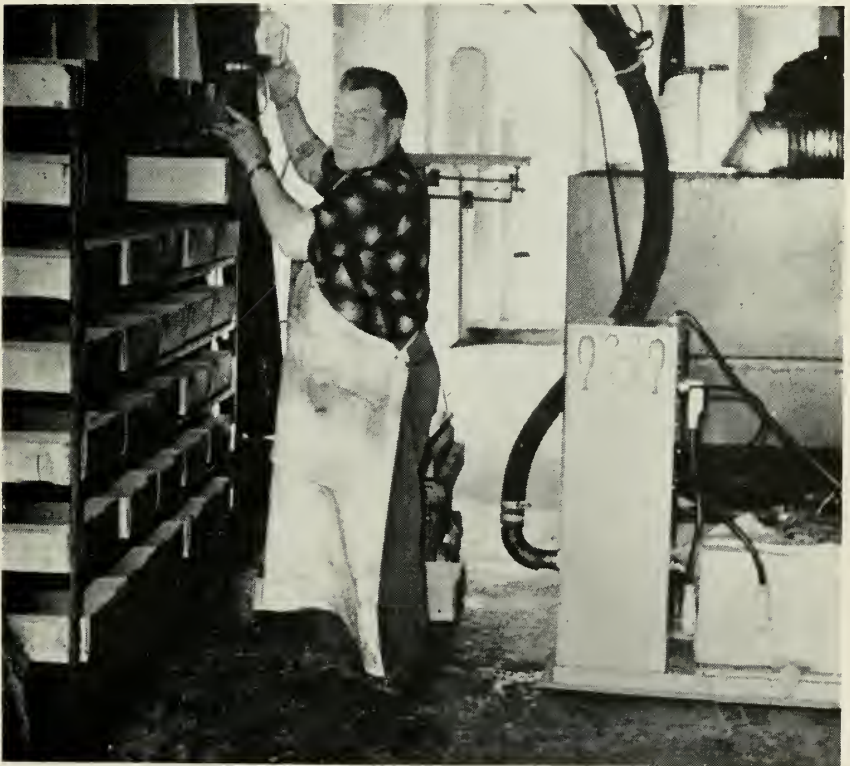
FIGURE 2. Method of filling boxes prior to freezing. Large grinder and storage hopper is in right background, pump and timing apparatus shown in right foreground. Photograph by E. A. Best, August, 1956.
